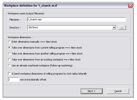
You may define a new blank or use the minimum/maximum values out of the milling program or use the result of a first simulation as input for a following simulation (see box "Workpiece dimensions", on the left side).
