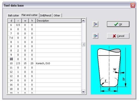
Choose from Spherical cutter, Cylindrical Cutter, Drill/Pencil or other tools out of the predefined tools and accept the selection, or enter the new values of a new tool
